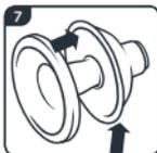
7. Push the soft, silicone cup into the widest part of the horn and smooth its lip evenly over the edge. Work your way all around the rim to make sure the cup fits smoothly, evenly and securely. The two dimples in the cup should be clear to allow air into the horn.
