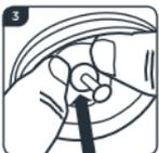
3. With two hands gently squeeze the bottom of the diaphragm over the ring in the base of the connector rod. The rod should be securely held by the diaphragm.
