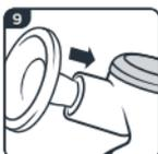
10. Insert the duck-bill valve. Gently squeeze the sides of the valve to make sure it opens.
