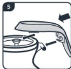
6. The handle should now freely move up and down and you should see the diaphragm lift up when you press the handle down.
