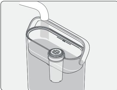
3. Fill filter hopper to the maximum level with cold water from the tap.
