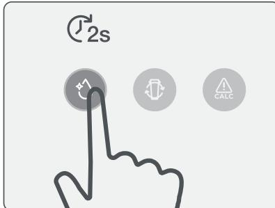
3. Press and hold the cleaning cycle button (L) for 2 seconds to start. If you need to pause, tap the cleaning button once and to restart tap the cleaning button again.
