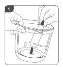
1. Slide the knife blade down over the shaft. WARNING! Handle the knife blade carefully as it is extremely sharp.
