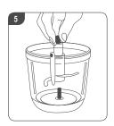
5. Make sure that the blade has stopped turning completely before removing the lid. Unplug the unit, remove the lid and remove the blender blade. Carefully pull the knife blade straight up. Empty the food from the bowl. Do not use the food blender bowl for storing food.
