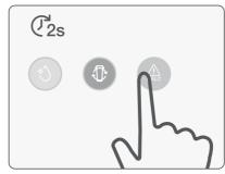
5. Press and hold descale button for 2 seconds. If you need to pause, press the button again. Press and hold the same button for 2 seconds if you need to cancel.
