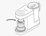
**8.** Remove the lid and place your bottle back on the stand. Press the Power button (N) again to dispense the remaining water.
