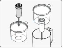
**4.** The filter is ready to fit into the filter hopper (C). Push downwards until it is positioned firmly.
