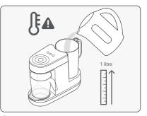
2. Add boiling water straight from the kettle into the water jug (D). The temperature warning light (L) will illuminate during the cleaning process.
