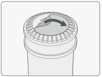
1. Remove the filter from packaging and remove the sticker from the top of the filter.
