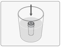
2. Submerge the filter in a bowl filled with cold tap water.
