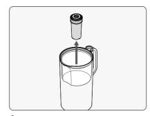
Remove the filter hopper and filter (always place them on a clean surface).
