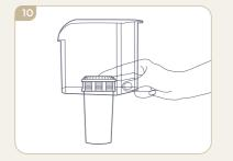
Remove the water hopper from the unit and fit the filter by pushing the white part through the base of the hopper until
