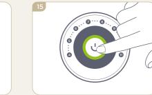
Press the start/stop button. A green light will flash and water will be dispensed to finish the cycle. Discard the dispensed water.
