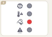
The water level low warning light will illuminate once the water has flushed through the system.
