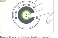
Press the start/stop button again. The red light will go out and the green light will flash whilst a volume of COLD FILTERED WATER is dispensed into your bottle to make up the remainder of the feed.
