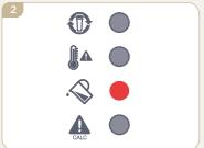
Plug in the unit, the water level low warning light will illuminate.
