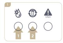
Press the cleaning mode button for 2 seconds to empty the tank (ensure a suitably sized container is under the dispenser to collect the water). Then press the filter volume reset button for 2 seconds to clear the memory.
