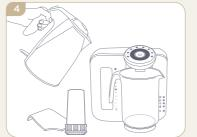
With the water hopper in place (but not the filter) fill the hopper with 1 litre of freshly boiled water - HOT WATER -
