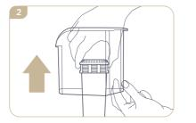
Remove the water hopper from the unit and then remove the filter by gently pushing the white part from the base past the 3 securing clips. Dispose of the old filter in general household waste.
