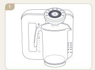
Place a container under the dispenser outlet to capture the water used to clean the system (ideally at least 1 litre capacity).
