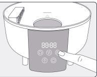
7. Select your desired function from the 4 function icon buttons. Your unit will automatically go on standby, if you don't select a new operation within 5 seconds. See 'How to use the different functions' for more information.
