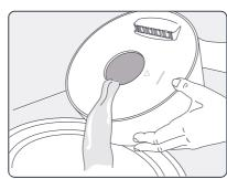
8. To drain any excess water away from the base, ALWAYS POUR SIDEWAYS, AWAY FROM THE AIR VENT.
