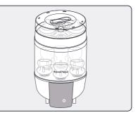
**5.** Place the lid on top. Double check that the lid fits securely onto the upper rack, without any gaps.
